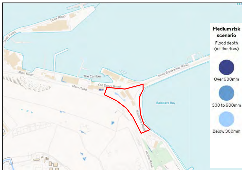
Figure 2.3 – Flood Risk from Surface Water
